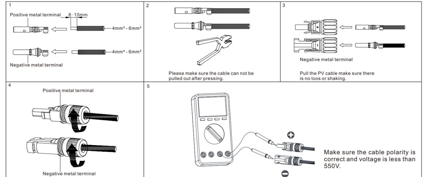
Make sure the cable polarity is correct and voltage is less than 550V.
